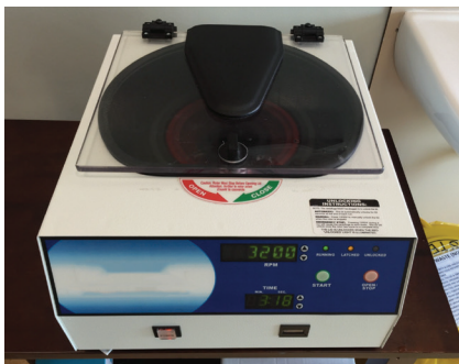
Figure 1. Tubes centrifuged at 3200 RPM for 10 minutes.
